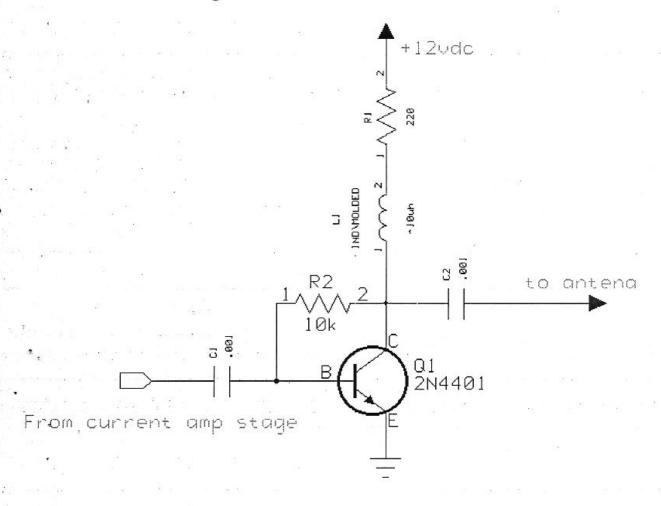
I built this thing right on the underside of the FM-10 kit, C1 is the cap that currently goes to the RCA ant jack, the 9k and the 220 ohm resistor have to be bought, note that if you cannot find 220 ohms you can make one by using 2 440 ohm resistors in parallel, and that a 10k will work in place of the 9k but yields poorer performance (-5%).
