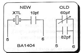
use a couple of capacitors. This has created nothing but problems for the kit builder. If you are having problems with stereo separation, you can solve this by lowering the value of C7 to 60pf (this usually works.) But messing with this mess you almost need a frequency counter so you can 'see' 19Khz at the test point.
