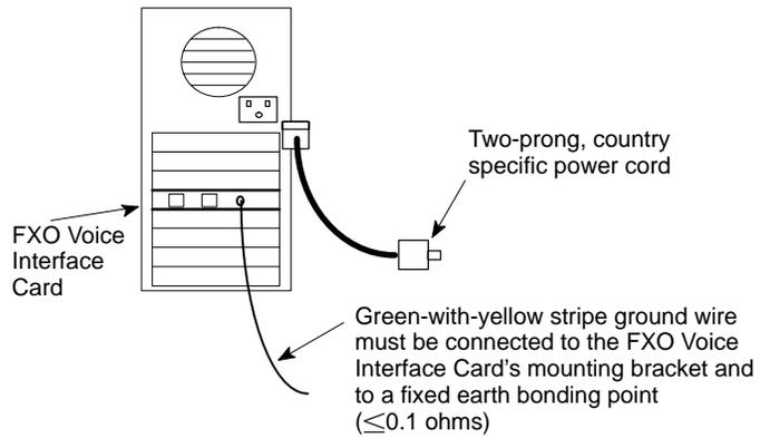
**Connection Using A Ground Wire Between the Voice Interface Card and A Fixed Earth Bonding Point (FXO Voice Interface Card *only*)**
