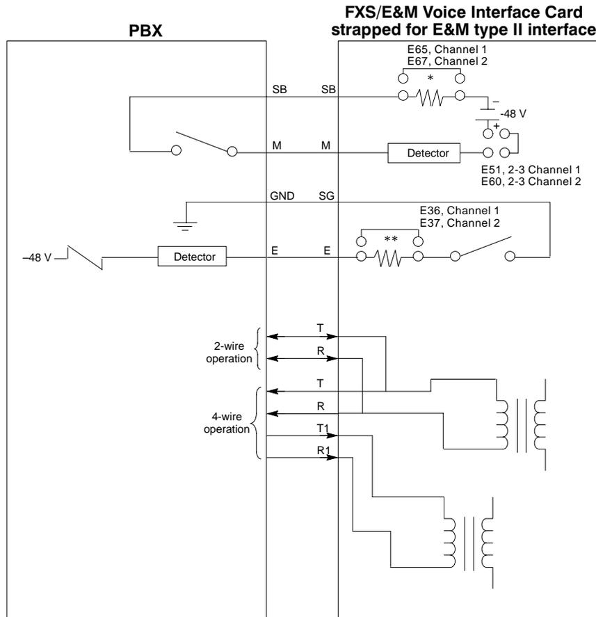
\* This jumper is installed only when SB lead loop resistance is too high due to long cable lengths.
