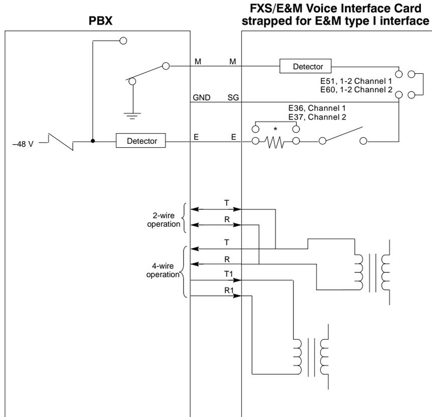
\* This jumper is installed only when E lead loop resistance is too high due to long cable lengths.
