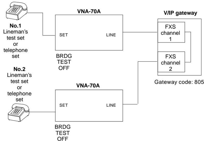
2. Lift the No.1 telephone set off-hook. Dial the gateway code and the No.2 channel number. The No.2 telephone set will ring.
