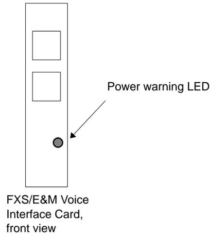
The LED should turn on momentarily as the Voice Interface Card is powering up. If the LED stays on continuously, this means the card is drawing too much current from the PC's +12V supply. If this happens:
