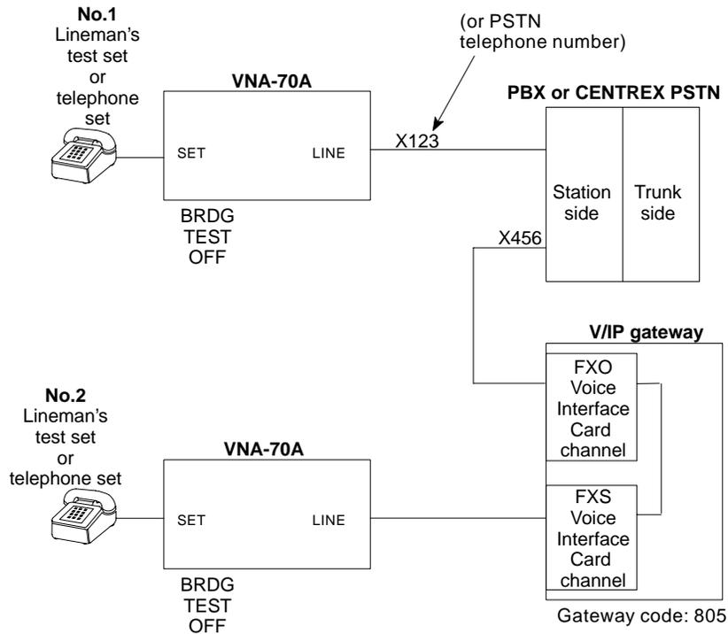
2. Place a call from PBX extension 123 to extension 456. To do that, lift the No. 1 telephone off-hook, wait for the dial tone from the PBX, then dial extension number 456. (In CENTREX PSTN applications, dial the published PSTN number.)
