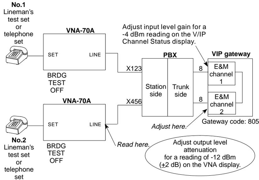
2. Select the first two E&M voice channels within the V/IP gateway to be adjusted. Set any additional voice channels to the busyout mode to insure that the test calls operate only through the channels under test.
