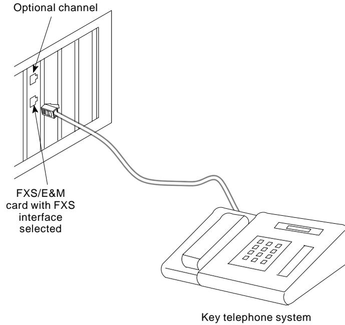
**Note:** The FXS interface is *not* intended for connection to the Public Switched Telephone Network.
