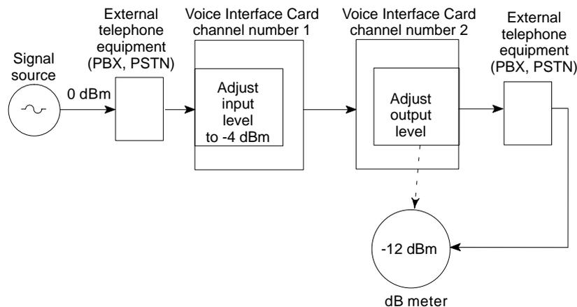
Next, the two voice channels remain connected as before, but the signal flow is reversed. What was previously the receiving voice channel now becomes the sending channel, and vice versa, and the adjustments are made in a reverse order.
