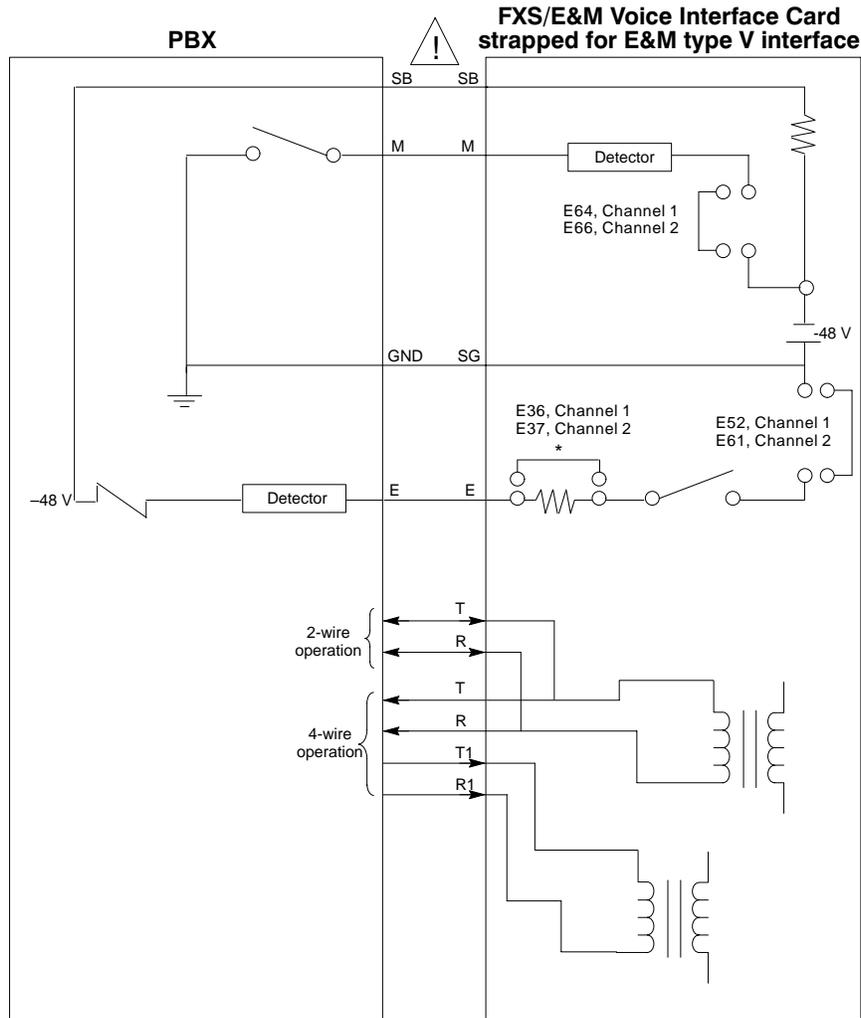
\* This jumper is installed only when E lead loop resistance is too high due to long cable lengths.
