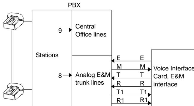
Audio is implemented on either a single pair of wires (2-wire) labeled T/R, or on two pairs of wires (4-wire) labeled T/R and T1/R1, as configured. When configured for 2-wire operation, the T/R pair is used for both transmit and receive. When configured for 4-wire operation, the T/R pair is used for transmit (output from the Voice Interface Card) and the T1/R1 pair is used for receive (input to the Voice Interface Card).
