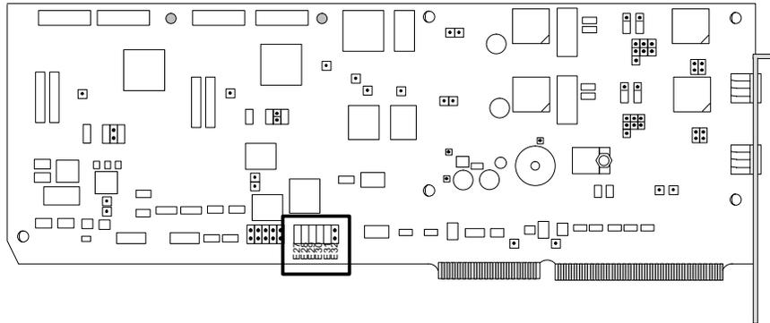
*FXO card: set the I/O port base address on jumpers E7 to E13:*
