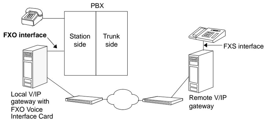
In the above example, at the local side, you would dial the local FXO station number and wait for a second dial tone. The local server's FXO channel will wait the number of cycles selected for the Number of Ring Cycles option, before providing a dial tone. This applies only to calls originating at the FXO side of the WAN; it does not affect calls received by the FXO channel.
