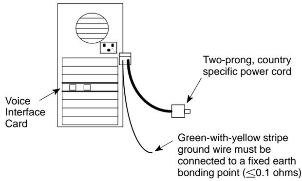
**Connection Using A Two-Prong Power Cord With Separate Ground Wire**
