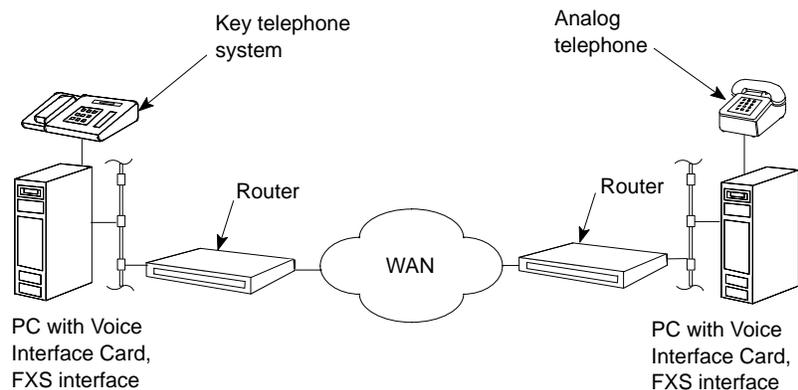
**Note:** The FXS interface is *not* intended for connection to the Public Switched Telephone Network.
