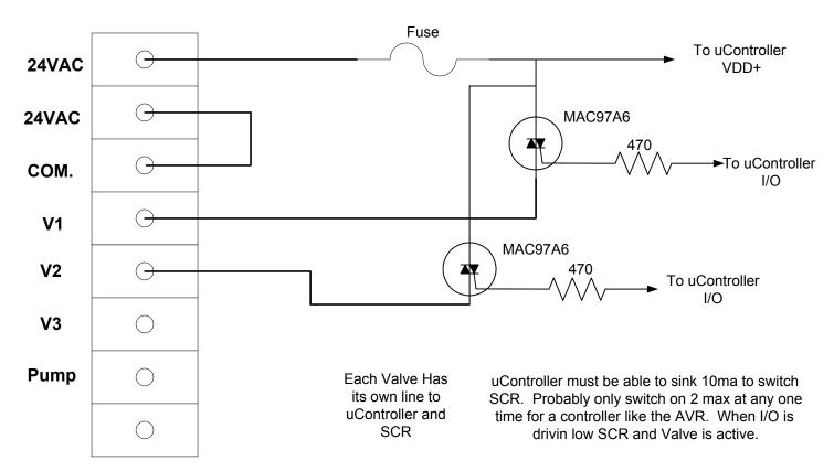
This design can control higher voltages than 24VAC, but I recommend using a photo SCR to switch dangerous voltages and current.
